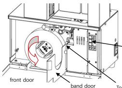
b. Close the band door and hold the end of the band, push it through the guide roller and assistance guide and then between the Idle roller and the main roller. Press the Automatic/Forward button, then the rollers will turn to move the band forward. At this point, allow the band to roll in automatically as shown in the diagram.
